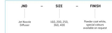
Holyoake Jet nozzle diffusers shall be of spun aluminium construction with a steel concealed mounting system. They shall be designed to supply large air quantities over large throws.
