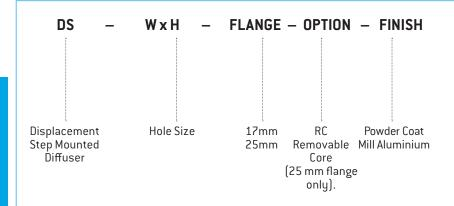
Displacement Step Mounted Diffusers shall be Holyoake Series DS. They shall be designed to mount into a supply plenum at floor level and to provide an even distribution of air flow at low velocity, thereby creating a draft-less environment. Pressure drop through the displacement diffusers will be such to provide balance within the supply plenum, while being low enough to generate very low noise levels.
