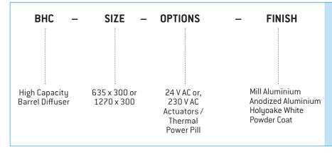
High Capacity Barrel Diffusers shall be Holyoake Series BHC. They shall be designed to be mounted into a supply plenum that may contain a number of BHC units, which will provide high capacity and long throw diffusion. Adjustment is available to change the vertical and horizontal throw and spread.
