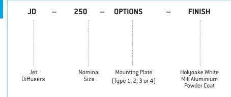
Circular Jet Diffusers shall be Holyoake Model JD constructed from spun aluminium cones. JD Jet Diffusers shall be capable of operating in either diffused, or jet air pattern configurations. The air patterns shall be achieved by rotating the cone assembly through 180 degrees. JD Jet Diffusers shall be complete with a mounting system suitable for wall, or ceiling applications.
