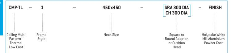
Ceiling Multi Pattern - Thermal Low Cost Louver Face diffusers shall be type CMP-TL. They shall be of Aluminium construction, with removeable cores. CMP-TL central cores, are complete with a vertical supply section controlled by a thermally actuated damper. Supply air is diffused horizontally below temperatures of 24°C and vertically with temperatures above 30°C.
