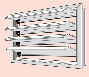
BDE shutters must not be installed with the axles vertical.
