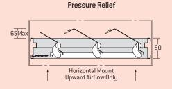
Channel Style Illustrated (Shown within ductwork)
