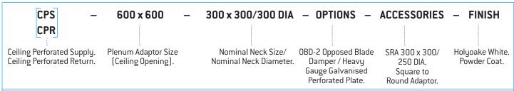
Ceiling Perforated diffusers shall be Holyoake Series CPS, or CPR and shall consist of an extruded aluminium frame with close mitred corners and 0.75 mm aluminium perforated face in an extruded aluminium sub-frame. The face shall be removable, by means of a separate mounting frame, which if used for supply air shall be furnished with field adjustable pattern control louvers and a galvanised steel plenum with duct connection. All shall be as manufactured by Holyoake.
