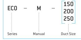
Ceiling diffusers shall be Holyoake Series ECO-M, manufactured from injection moulded tough U.V. stabilised and fire rated engineering polymer, in self coloured white as standard. Series ECO-M shall have the ability to regulate the airflow via an adjustable central cone.
