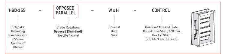
Balancing Dampers shall be of extruded aluminium construction. Frames shall be suitable for duct flange mounting. Blades shall be fixed to 11 mm hexagonal shafts held by two piece acetal self lubricating bearings, with outer shells fluted to prevent rotation.
