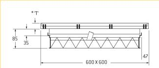
\* Dimension 'T' (Tile thickness) must be specified at time of order, between limits of 50 and 25mm. Where 'T' is less than 32mm, continuous support is required along all four sides to maintain the concentrated load bearing strength.
