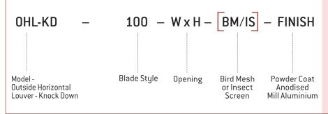
OHL-KD (Knock Down) Outside Horizontal Louvers shall be manufactured from aluminium extrusion and are supplied in Kit Form for on site assembly, by others. The louver blades shall be sight proof, complete with two water stops and may be provided in a powder coat finish, with Bird Mesh, or Insect Screen.
