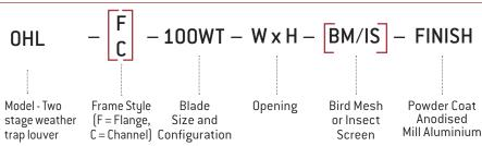
Horizontal Outside weather trap louvers shall be of extruded aluminium construction with 100mm front blades fixed at their ends and complete with second stage blades at the rear. The bottom louver shall overlap the frame and the structure shall be designed to withstand a wind load of 95 kg/m2.
