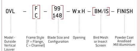
Vertical Outside Louvers shall be of extruded aluminium construction with blades fixed at ends with stainless steel screws into a mitred and mechanically locked extruded aluminium frame. Intermediate blade stabilizing spacer clips shall be fitted where blade length exceeds 900mm and the structure shall be designed to withstand a wind load of 95kg/m².
