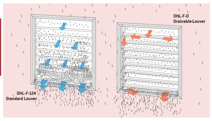
Holyoake Industries Model OHL-D offers an alternative concept in horizontal outside louvers. The drainable blade louver offers excellent water penetration performance.
