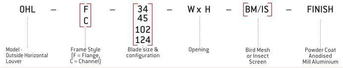
Horizontal Outside Louvers shall be of extruded aluminium construction with 100 mm blades fixed at their ends with stainless steel screws into a welded aluminium frame. The bottom louver shall overlap the frame and the structure shall be designed to with stand a wind load of  $95~{\rm Kg/m^2}$ .
