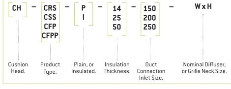
Holyoake Cushion Head boxes shall be constructed from galvanised steel and be complete with suitably sized galvanised steel connection spigots and accessories, as appropriate. Optional black polyester insulation, 14, 25, or 50 mm thick can be incorporated.
