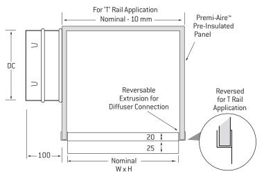
The Premi-Aire™ range adapts ceiling swirl, multi pattern, square neck diffusers, return grilles, linear diffusers and other applications to a side or top entry, round, oval or square/ rectangular spigot connection/or proprietary Duct Flange connecting arrangement.
