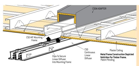
\*Note: Do NOT fix plaster board to ceiling battens closer than 300mm of mounting frame.
